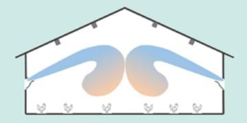
For floor housing, the AeroWing can be installed at a low height, since the air throw is independent of the roof slope. An additional advantage of this is that obstacles at roof height, such as roof trusses, lighting or winch-suspended feed and water lines, do not affect the air distribution.
