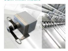
The EGM motors have been specially developed to control air intake systems in intensive livestock buildings. The EGMs are fitted with robust brushless 24V motors with a tractive force of 100 and 250 kg respectively. As standard, the EGM series is supplied with a cable drum and it is also available with a 0-10V control signal or potentiometer feedback.
